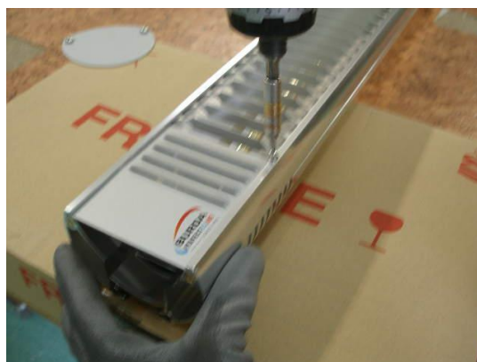
2.unscrew a protection screw
