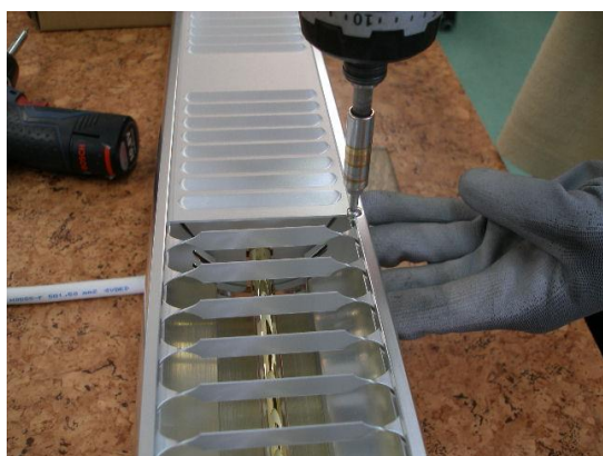
3. unscrew a protection screw
