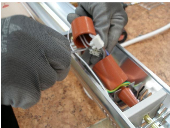
11. disassemble the emitters' cables
