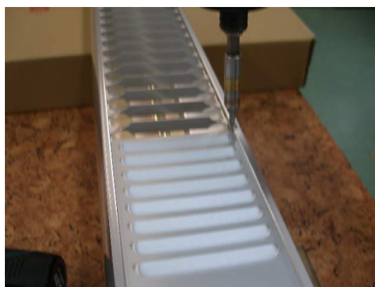
4. unscrew a protection screw
