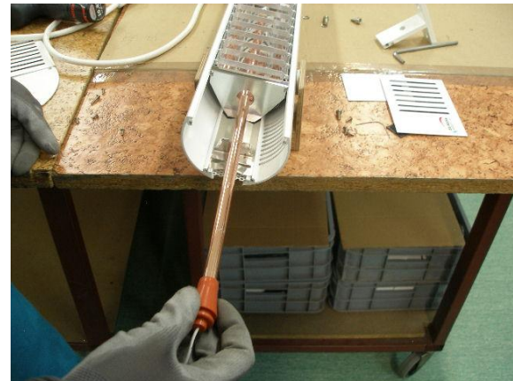
18. Dismount an emitter from a heater
