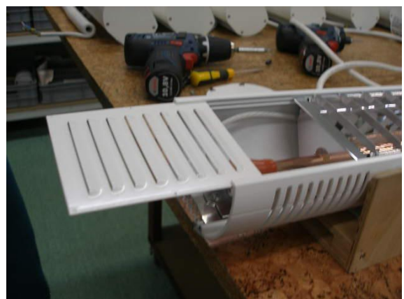
12. Dismount the second front element
