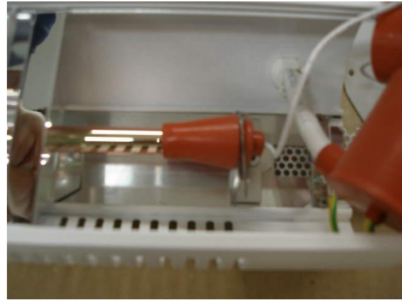
16. Dismount a spring from the second side.
