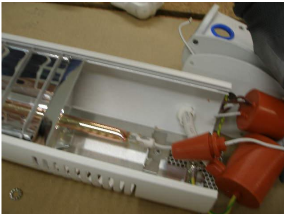
17. Dismount sealing of the emitter
