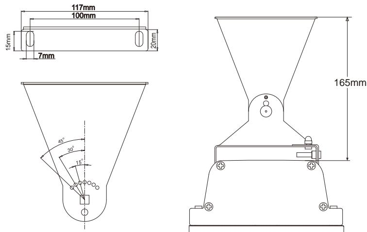
4. The correct installation process, as per the diagram above, select the location on the ceiling by locating the stud or structural beams to ensure secure fastening of the device, whilst observing the minimum clearances from the floor and other objections.
