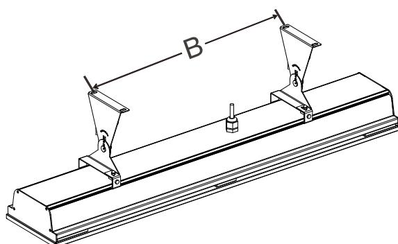
6. Set the adjustable angle mounting brackets to desired angle and fasten brackets by spanner
