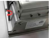
3. Remove the 4 screws on the left cover, as shown below.
