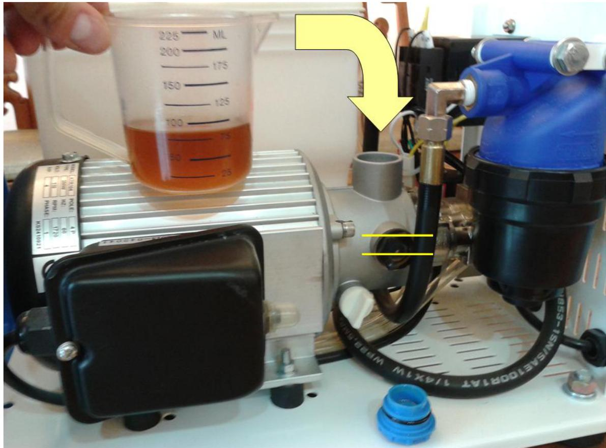
I have attached a labeled photo to help explain how to measure the oil and where to fill. Also, when looking into the oil window the level should be within the two yellow lines. Sometimes it helps to shine a flashlight into the top so the oil level can be seen more clearly in the window.
