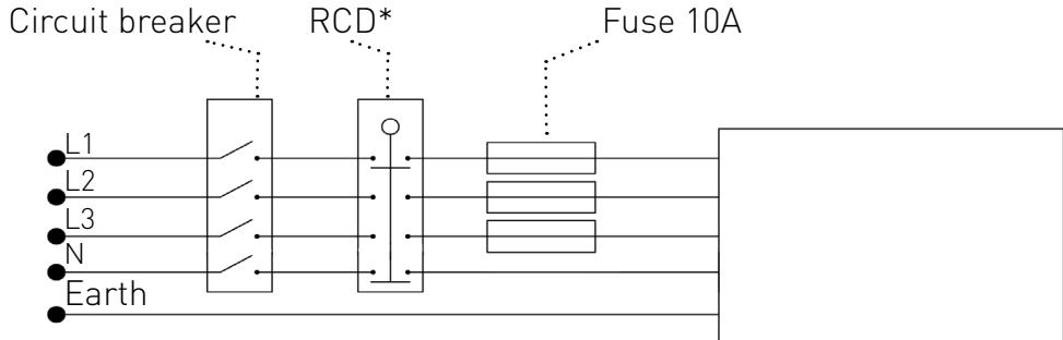
If the product is used indoors, it must be controlled by a chronothermostat. To control a product with three-phase connections with a single-phase chronothermostat, you will need a remote control switch and connect everything following the diagram below.
