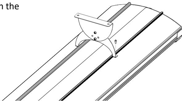
The support to be fixed to the wall presents a series of holes that allow to fix the heater in different positions.
